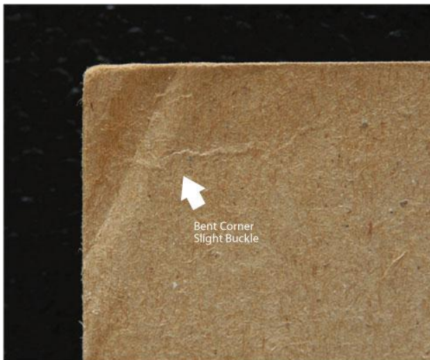
Corner Bent, Slight Buckle
