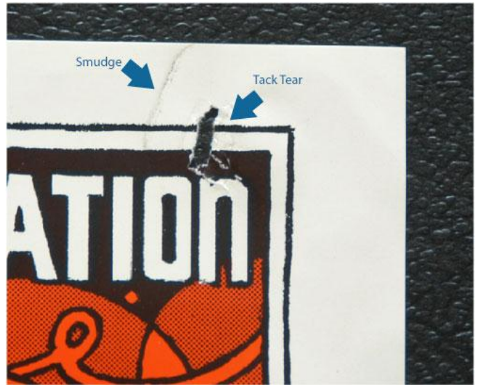
Tack Hole Tear
