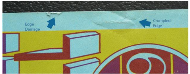
Edge Damage and Crumple
